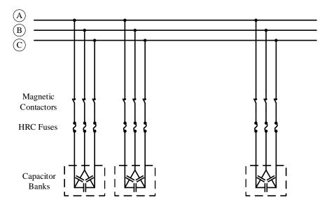
Figure 2.17: Circuit diagram of PFI plant.
