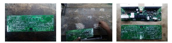
Figure 4.2: Soldering components onto the double layer PCB.
