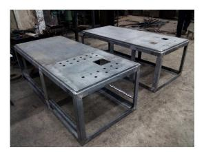
Figure 2.3: Frames for Switchgears.
