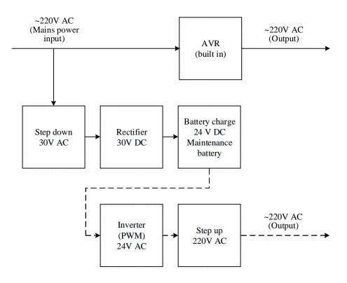
Figure 4.1: Block diagram of IPS (also of UPS).
