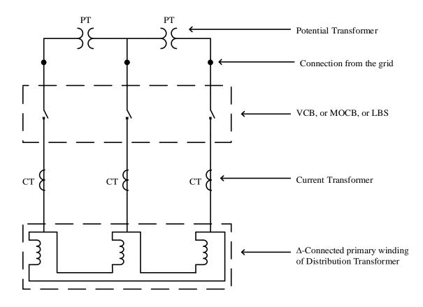
Figure 2.5: Circuit diagram of HT Switchgear.
