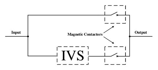
Figure 3.6: Connection of IVS with the magnetic contactors.
