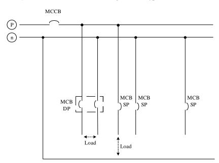
Figure 2.20: Circuit diagram of a typical DB.
