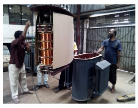
**Figure 2.15:** *Transformer being mounted inside the tank.*
