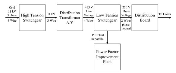
Figure 2.1: Sequence of the components as these appear in a power system.
