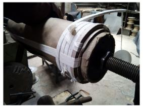
Figure 2.11: Making of LT winding.
