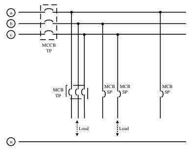
Figure 2.2: Circuit diagram of LT Switchgear.
