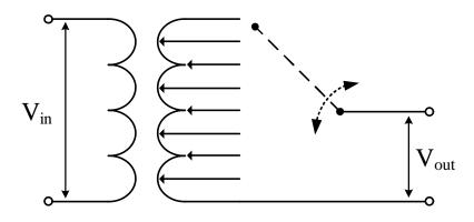
Figure 3.1: Circuit diagram of AVR.
