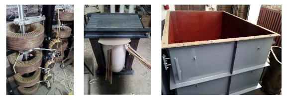
Figure 3.7: Variacs, transformers and tank for IVS.
