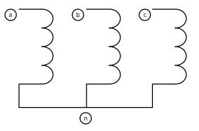
Figure 2.7: Y-connected secondary winding.
