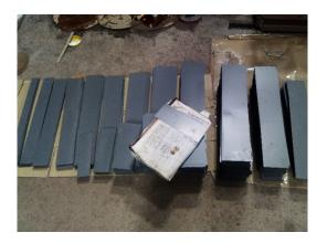
Figure 2.8: CRGO sheets cut as per the design.
