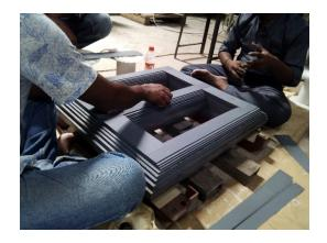
Figure 2.9: Assembling the transformer core.
