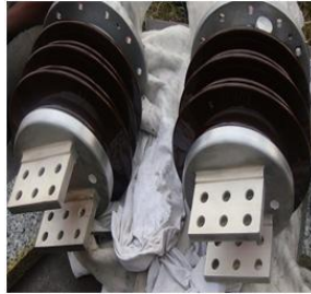
Figure 4-4: Bushing of transformer
