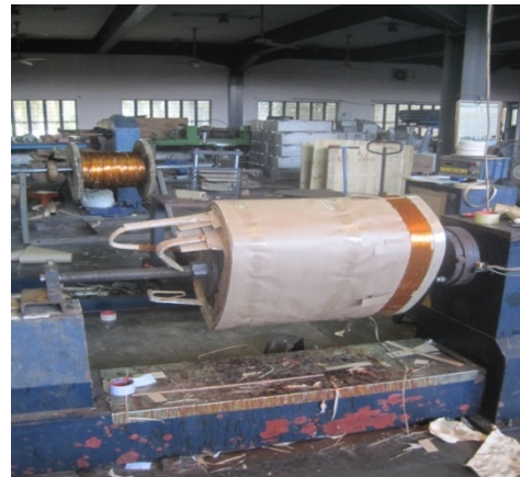
Fig5.6: Repairing a x-former with isolating paper
