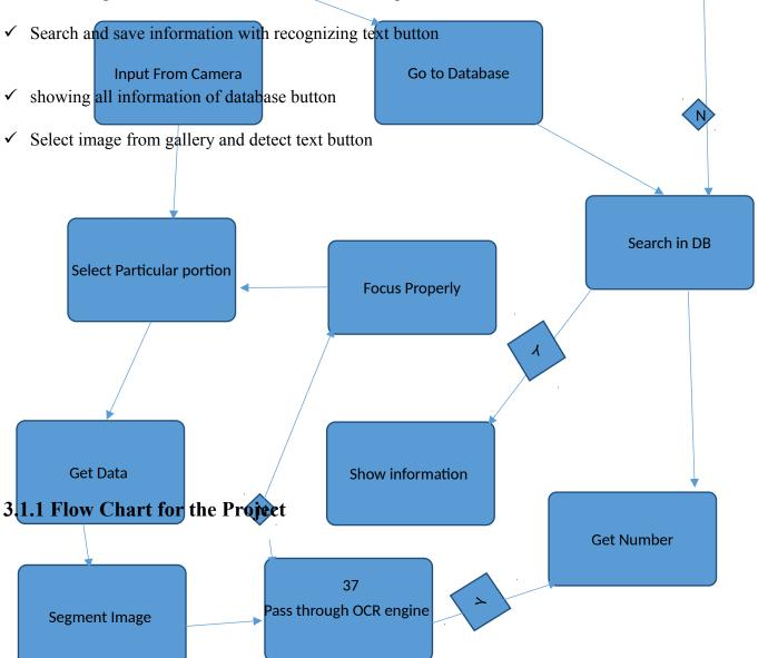
Figure: Flow chart for Nameplate Text Detector using Android Application.
