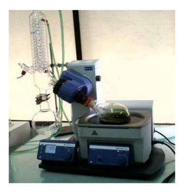
Figure 3.1: Drying of extract using rotary evaporator.
