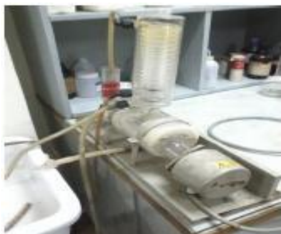
Fig 3.1: GENRISTO Distill Water Plant
