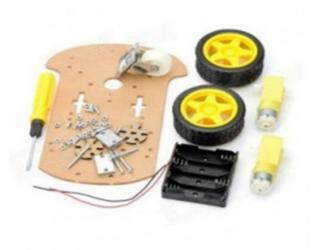
This robotic chassis kit contains of an acrylic base with two gear motors, two compatible wheels, a ball caster, and other accessories.
