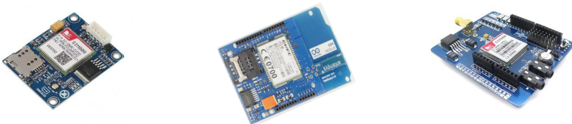
Fig: Different Types of GSM Shield
