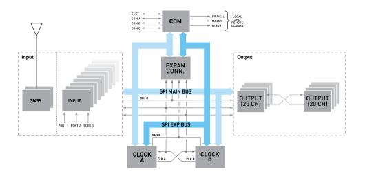
Figure 5.2: SSU 2000/2000e block Diagram
