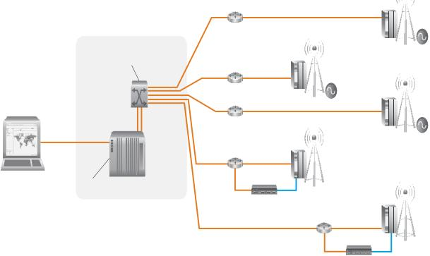
Figure 7.1: IEEE 1588 (PTP) Grandmaster Server Cards provide synchronization traceability over Ethernet to PTP clocks in remote base station.
