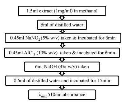
Figure 3.4: Schematic diagram of preparation of blank solution
