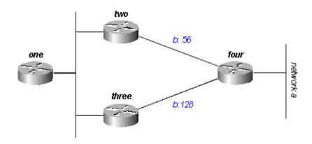
Fig 6: Load balancing scenario
