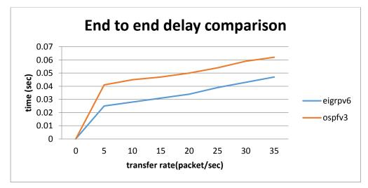
Fig 12: End to end delay comparison between OSPFv3 and EIGRPv6
