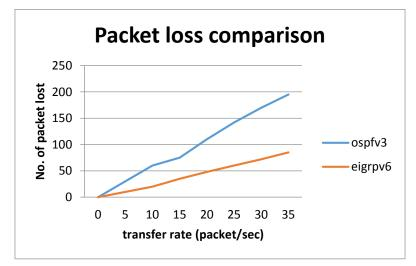
Fig 11: Packet loss comparison between OSPFv3 and EIGRPv6
