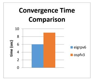
Fig 13: Convergence time comparison between OSPFv3 and EIGRPv6
