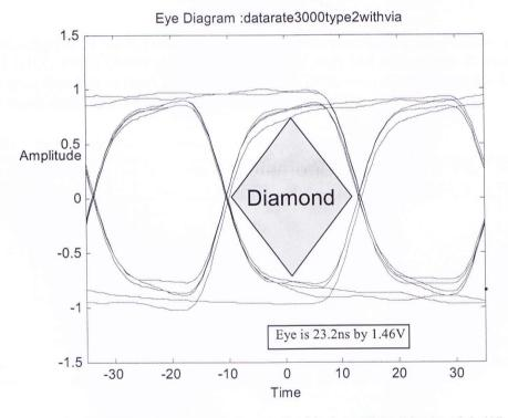
Figure 22: Eye diagram of Design type 2 with via at 3GHZ. Line length is 13".
