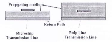
Figure 10: Types of Transmission Line
