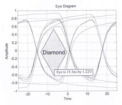
Figure 27: Eye diagram of Design type 3 with via at 1GHZ. Line length is 24".
