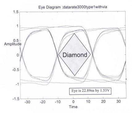
Figure 21: Eye diagram of Design type1with via at 3GHZ. Line length is 13".
