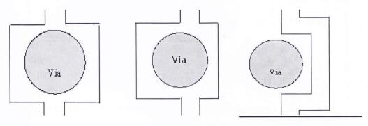
Figure 14: Via configurations, left - type 1, center - type 2, right - type 3.
