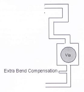
Figure 13: Extra length compensation to omit impudence mismatch
