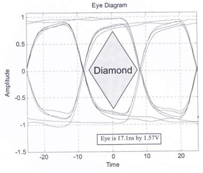
Figure 24: Eye diagram of Design type 3 without via at 1 GHZ. Line length is 13".
