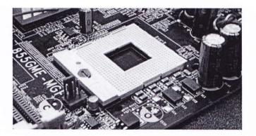
Figure 9: Socket on a printed circuit board.
