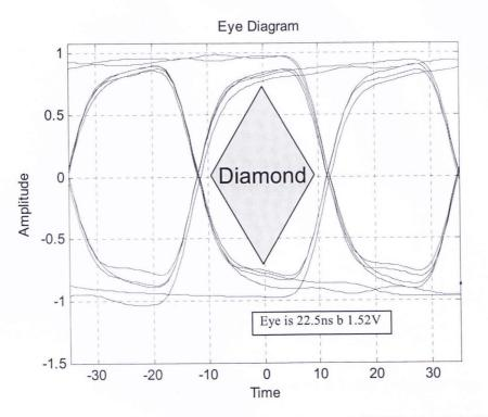
Figure 29: Eye diagram of Design type 3 without via at 3 GHZ. Line length is 13".
