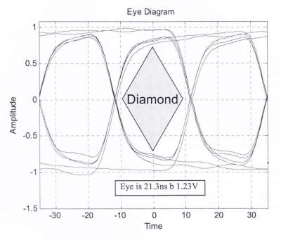
Figure 31: Eye diagram of Design type 3 without via at 3 GHZ. T-line is 24" long.
