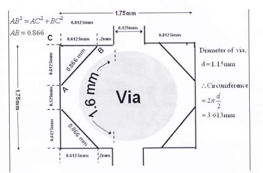
Figure 15: Measuring mutual capacitance of type 1 via configuration
