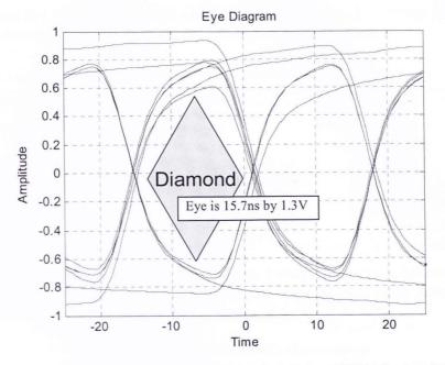
Figure 26: Eye diagram of Design type 3 without via at 1GHZ. Line length is 24".
