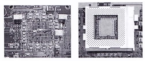
Figure 16: Surface mounted components and a CPU Socket of a Printed circuit board
