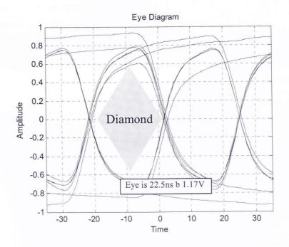
Figure 30: Eye diagram of Design type 3 with via & data rate is 3 GHZ. T-line length is 24" long.
