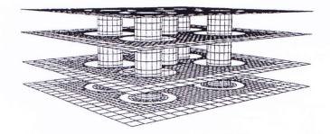
Figure 5: 3D view of vias in multiple layer
