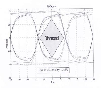
Figure 25: Eye diagram of Design type 3 with via at 1 GHZ. Line length is 13".
