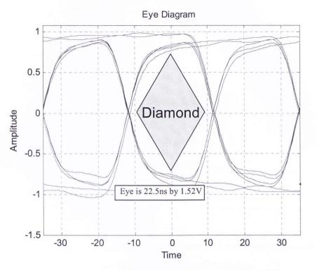
Figure 20: Eye diagram of Design type 3 without via at 3GHZ. Line length is 13".
