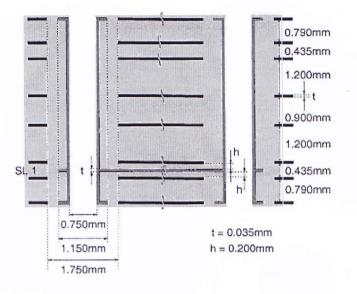
Figure 12: Configuration 8 layer printed circuit board through vias
