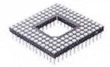
Figure 8: PGA type package
