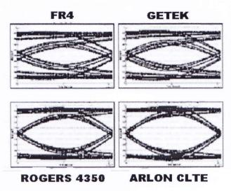
Figure 4: Effect on data eye of high frequency losses in printed circuit board
