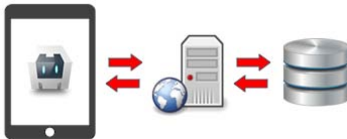
Fig 2.5 : Phonegap high-level application architecture
