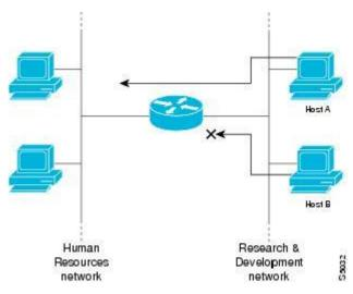
Figure 3.2 Using Traffic Filters to Prevent Traffic from Being Routed to a Network
