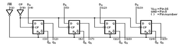
Fig 3.5.2: Logic Diagram of 4-bit parallel register
