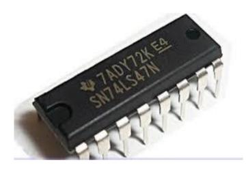
Fig 3.4.3: BCD to 7-segment display decoder driver
