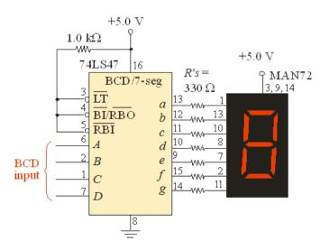
Fig 3.4.4: Connection with 7-segment display
