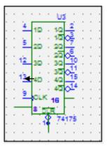
Fig 4.7.2: 4-bit parallel register(74LS175)
