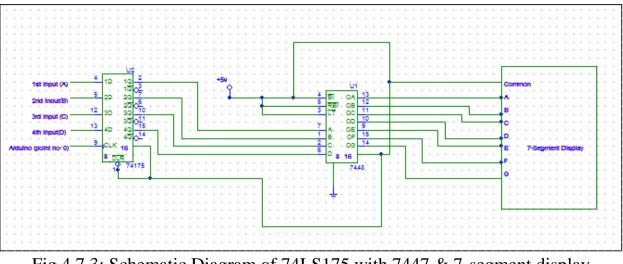
Fig 4.7.3: Schematic Diagram of 74LS175 with 7447 & 7-segment display
