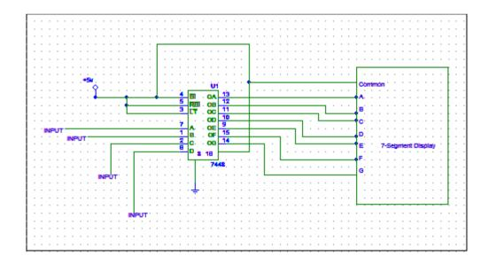
Fig 4.4.3: Schematic Diagram of connection between 7-Segment Display & 7447
