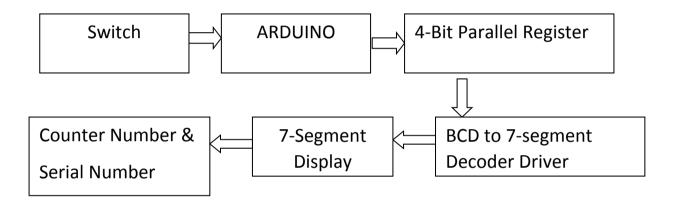
Fig 4.2: Block Diagram
