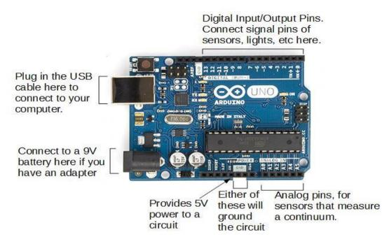
Fig 3.1.3: Arduino-UNO R3 Board
