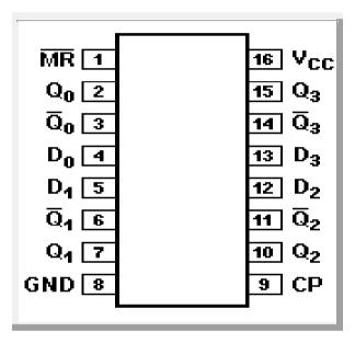
Fig 3.5.3: 4-bit Parallel Register
