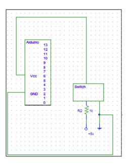
Fig 4.6.3: Schematic Diagram of Switch With Arduino
