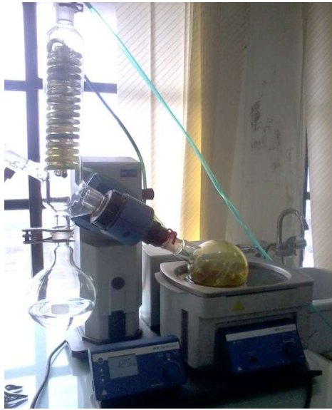
Figure-24: Evaporation of methanol by Rotary evaporator
