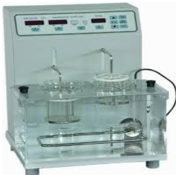
Fig 3.6: Disintegration Tester (Electrolab India)
