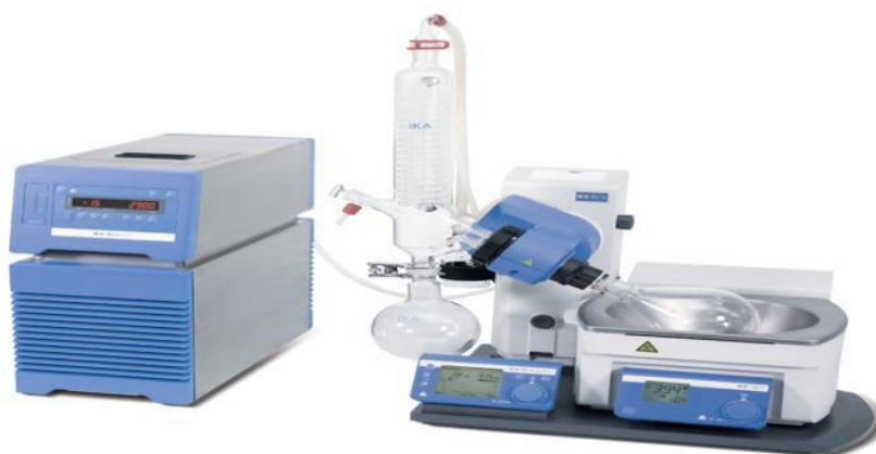
Figure 3.1: Drying of extract using rotary evaporator
