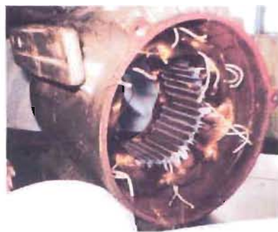
Figure 2.39: A re-wound motor
