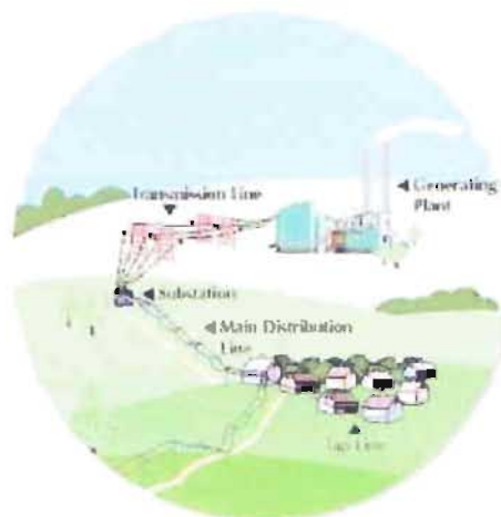
Figure 4.2: Power generation and distribution network
