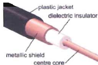
Figure 4.17: Co-axial cable model
