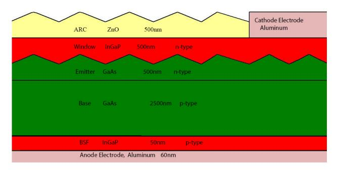
Figure-3.4: Structure of textured solar cell.
