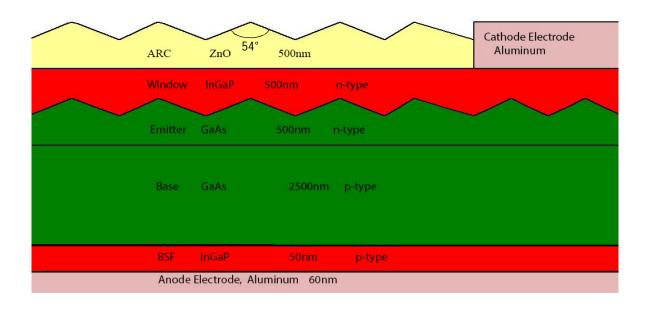
Figure 2.2: Textured single junction solar cell.
