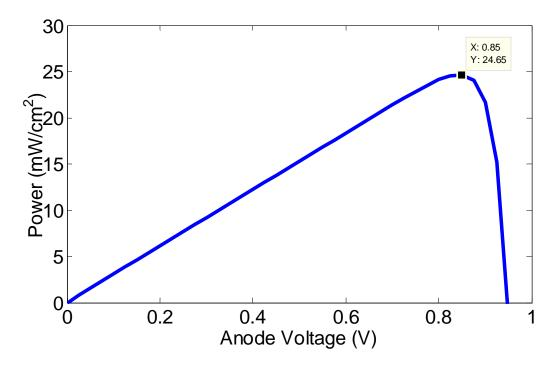
Figure-3.7: Power versus anode voltage of textured solar cell.
