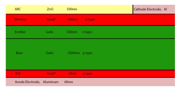
Figure-3.2: Structure of Non-textured solar cell.
