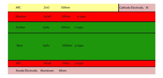
Figure 2.1: Non-textured single junction solar cell.
