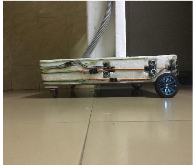
Figure 3.8: Ultrasonic sensor right view
