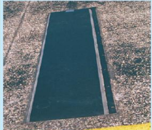
A weigh-in-motion speed and axle detection pad.
