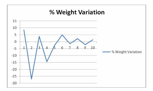
Figure 3.26: Graph of the percentage weight variation of 3 hour exposed samples.
