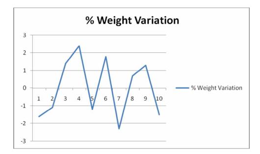
Figure 3.20 : Graph of the percentage weight variation of 3 hour exposed samples.
