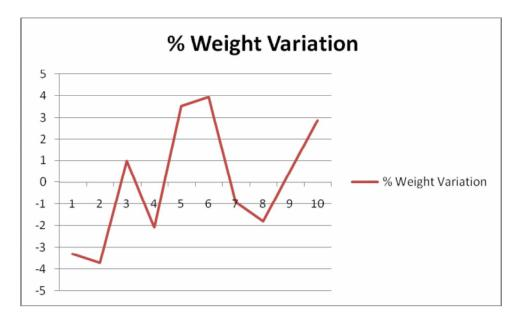
Figure 3.28: Graph of the percentage weight variation of 9 hour exposed samples.
