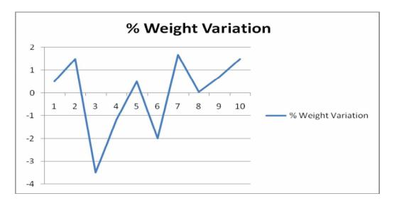
Figure 3.10 : Graph of the percentage weight variation of 9 hour exposed tablet samples in summer season
