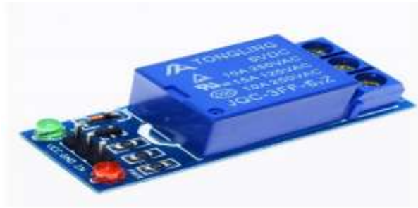
Fig 3.2: 1-Channel Relay Module [15]
