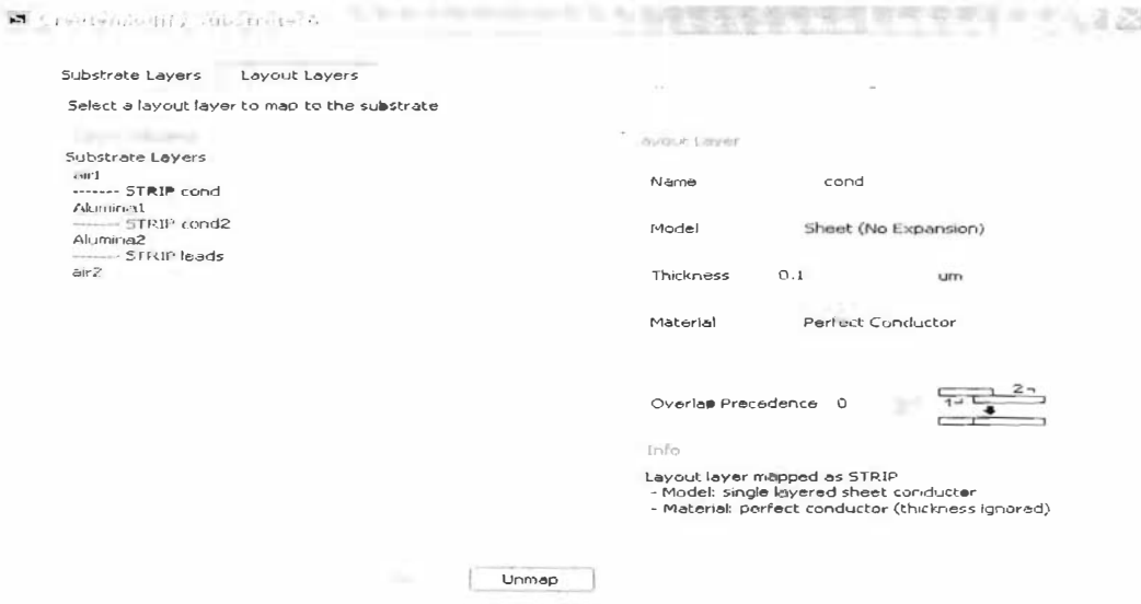
Figure 27: The ADS Layout layers window showing the declaration parameter while designing capacitor
