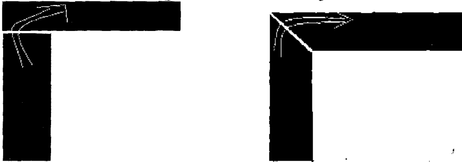
Figure 23: Normal Core Cutting and auto Core Cutting
