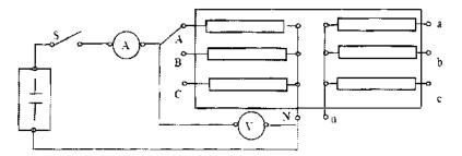
Fig 15: Circuit Diagram of Winding Resistance Measurement.
