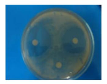
Fig.2.1 Zone of inhibition of sample and standard
