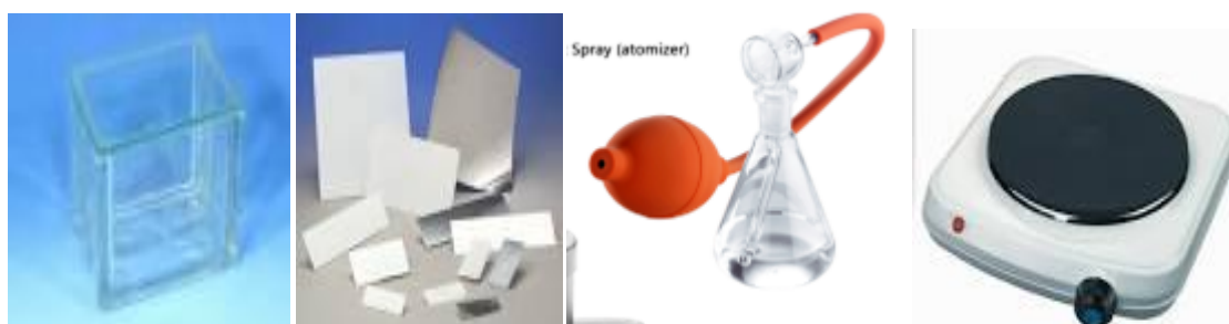
Fig 17: TLC tank (1), TLC Plate (2), Spray bottle (3), Hot plate (4)
