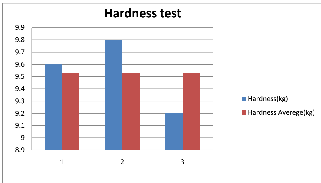
Figure 4.52: Column showing the difference of Hardness (kg) with Hardness Average (kg) of the tablets of 35 days sample
