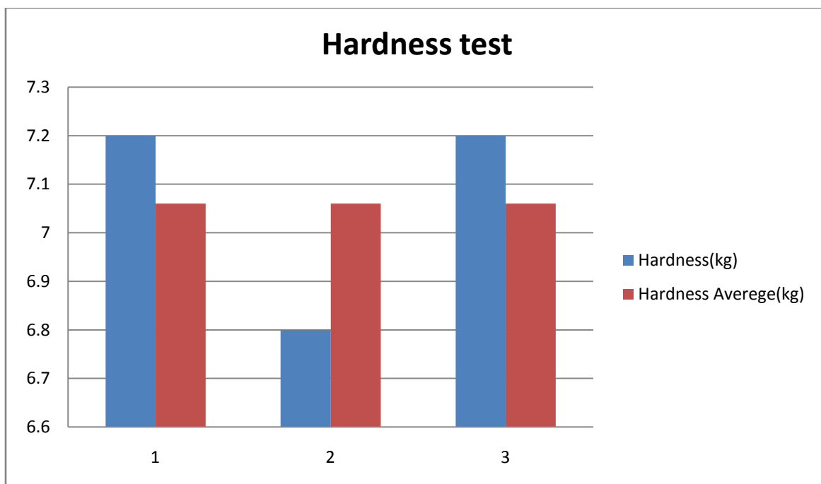
Figure 4.44: Column showing the difference of Hardness (kg) with Hardness Average (kg) the tablets of three hour sample of 40 watts electrical bulb
