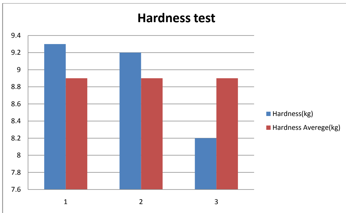
Figure 4.47: Column showing the difference of Hardness (kg) with Hardness Average (kg) of the tablets of three hour sample of sunlight
