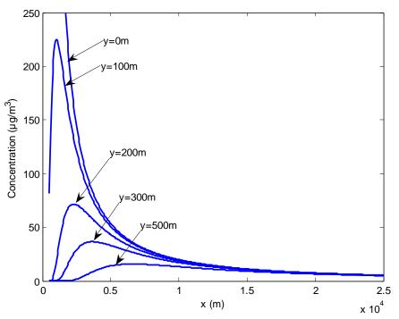
Fig. 4.5 Variation of the best case concentration with the increase of distance x for different values of y.
