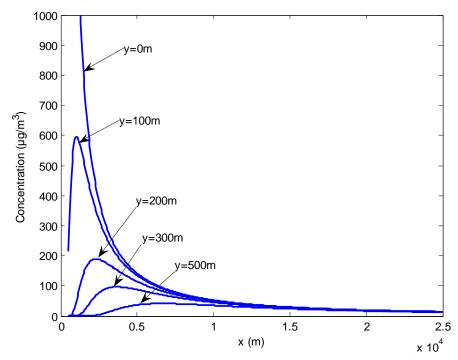
Fig. 4.6 Variation of the worst case concentration with the increase of distance x for different values of y.
