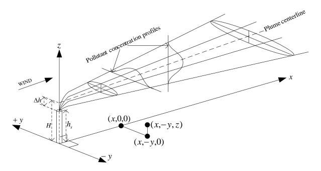
Fig. 3.1 Coordinate system for the Gaussian Plume Dispersion model.
