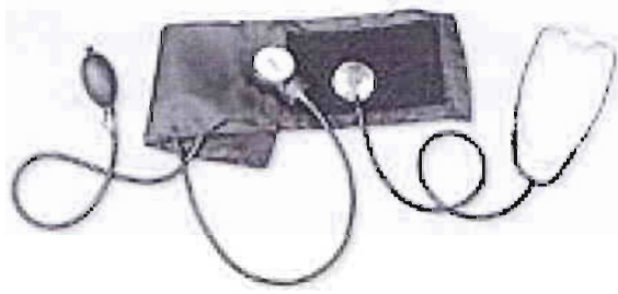
Fig: Conventional (mechanical) sphygmomanometer with aneroid manometer and stethoscope, used to measure blood pressure
