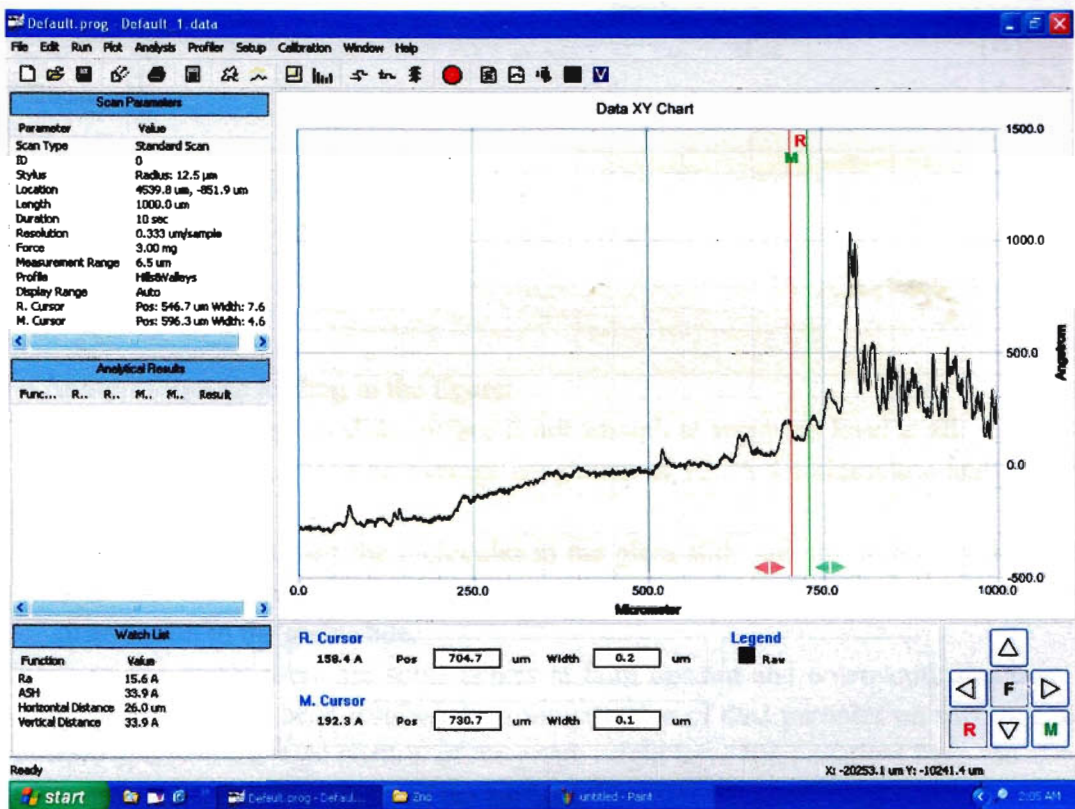
Fig8.1: Observing non-uniformity of a glass slide for aluminum.
