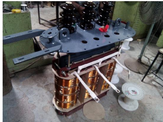
**Figure 2.13:** *After windings configured and tap changer installed.*
