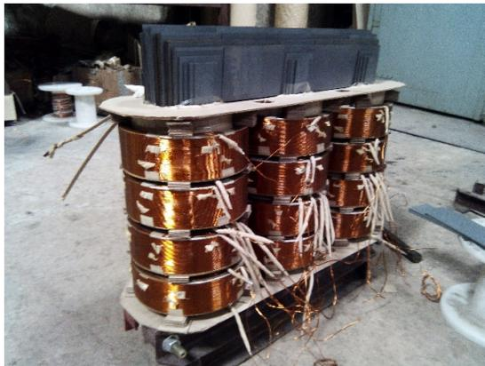
**Figure 2.12:** *The core after the windings are put.*
