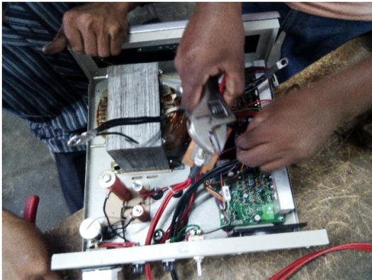
**Figure 4.3:** Construction of IPS.
