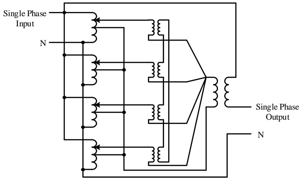
**Figure 3.5:** Circuit diagram of a single phase of IVS (with 4 variacs).
