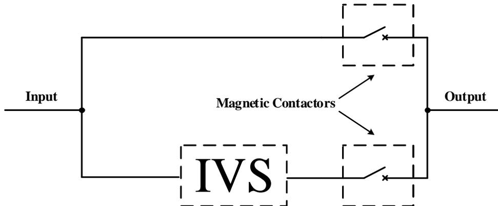
**Figure 3.6:** Connection of IVS with the magnetic contactors.
