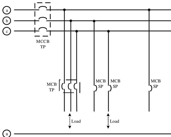
**Figure 2.2:** Circuit diagram of LT Switchgear.
