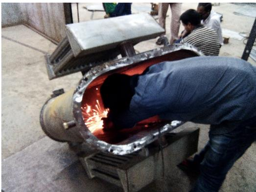
**Figure 2.14:** *Welding the tank.*
