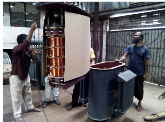
**Figure 2.15:** *Transformer being mounted inside the tank.*
