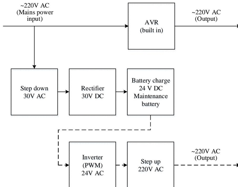
**Figure 4.1:** Block diagram of IPS (also of UPS).
