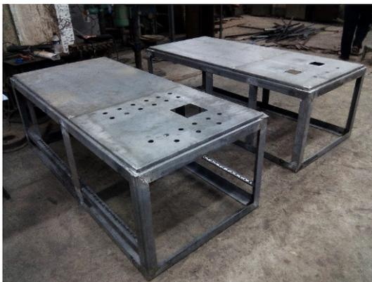
**Figure 2.3:** *Frames for Switchgears.*
