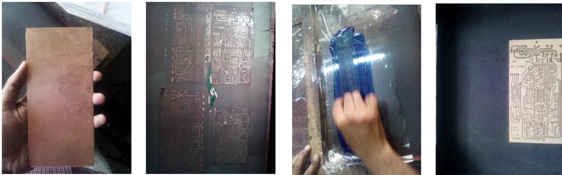
**Figure 3.2:** *Different steps of making a single layer PCB.*
