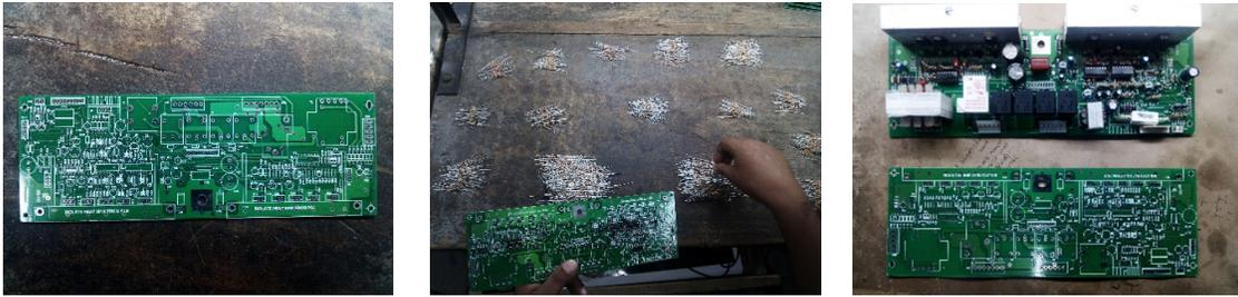
**Figure 4.2:** Soldering components onto the double layer PCB.
