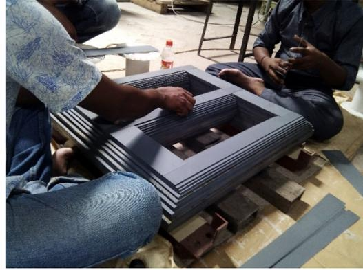
**Figure 2.9:** Assembling the transformer core.
