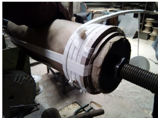
**Figure 2.11:** Making of LT winding.
