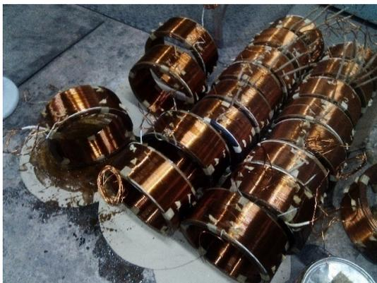
**Figure 2.10:** HT coils after turns are complete.
