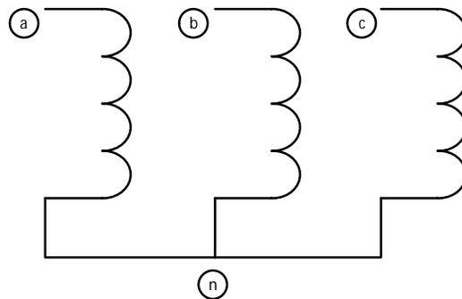
**Figure 2.7:** Y-connected secondary winding.
