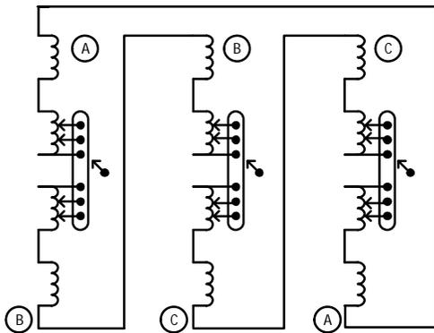
**Figure 2.6:**  $\Delta$ -connection of HT Winding with taps.
