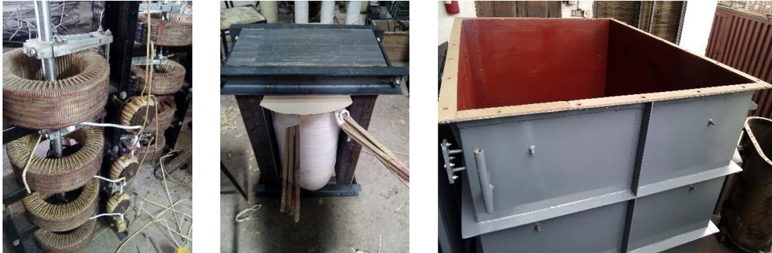
**Figure 3.7:** *Variacs, transformers and tank for IVS.*
