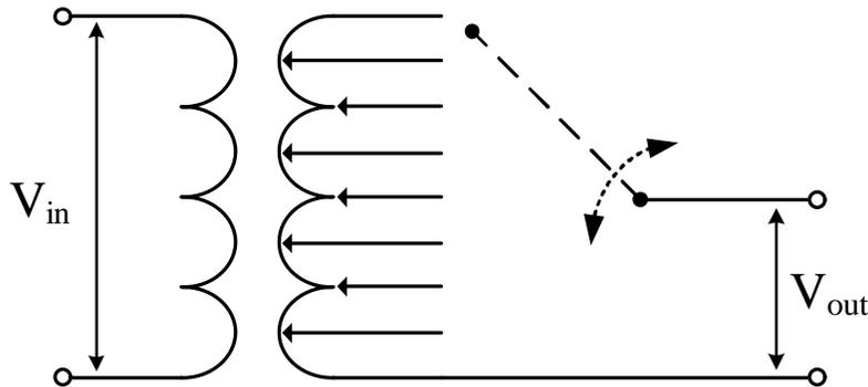
Figure 3.1: Circuit diagram of AVR.
