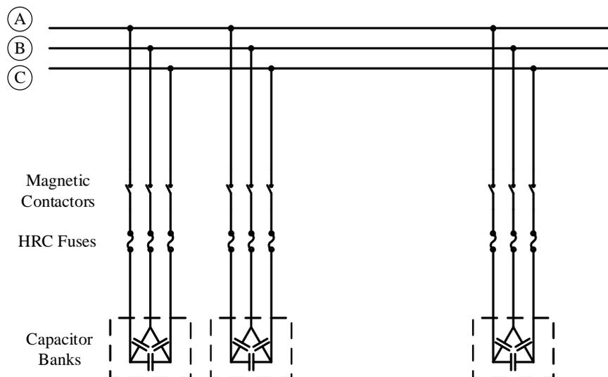
Figure 2.17: Circuit diagram of PFI plant.
