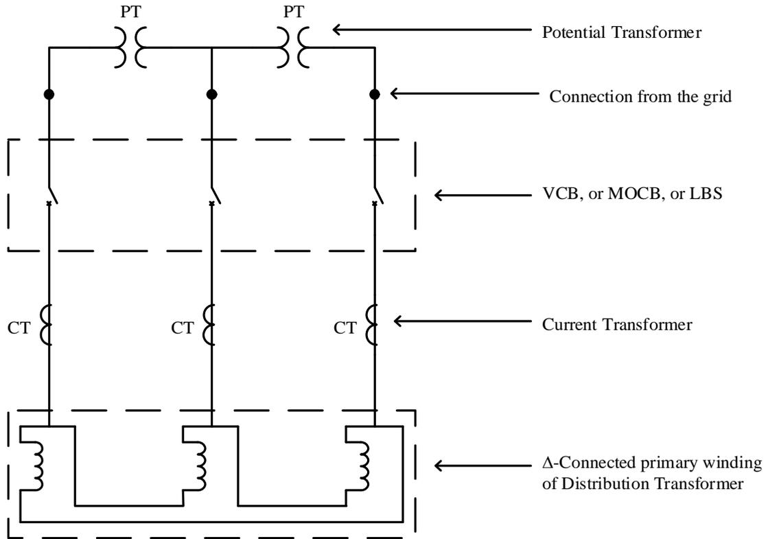
Figure 2.5: Circuit diagram of HT Switchgear.
