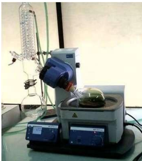
Figure 3.1: Drying of extract using rotary evaporator.
