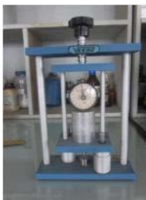
Figure 3.3: Hardness tester (Veego, India)
