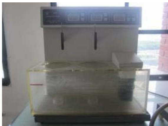
Figure 3.4: Disintegration tester (Vanguard Pharmaceutical Machinery INC)
