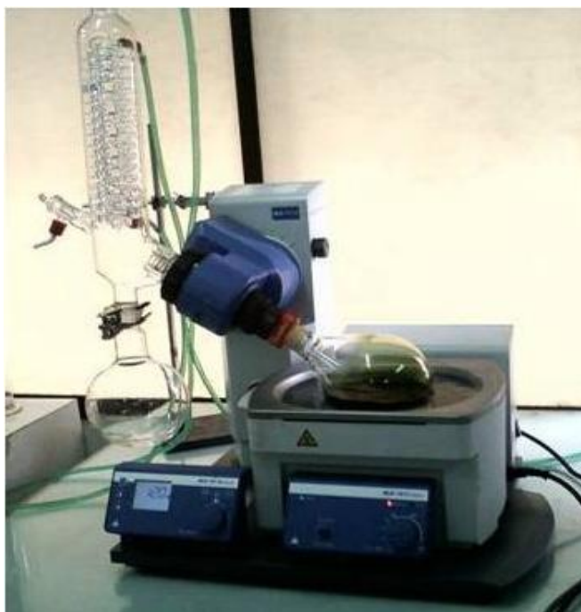
Figure 3.1: Drying of extract using rotary evaporator.
