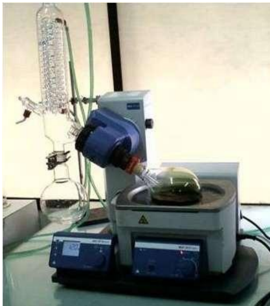
Figure 3.1: Drying of extract using Rotary evaporator
