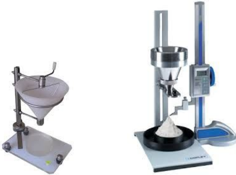
Figure 1.2: [Left to right] A set up of funnel with stand and measuring angle of repose
