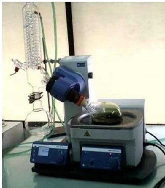
Figure 3.1: Drying of extract using rotary evaporator.
