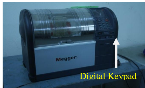
Figure 5.1: Dielectric Oil Test Module of EGCB
