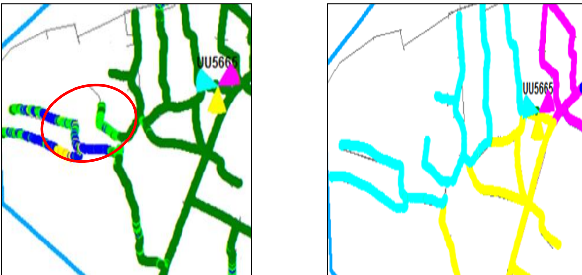
Fig3.4: Poor coverage explanation due to long distance call
