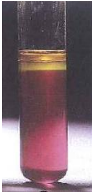
Figure 3.7: Preparation of test tubes for MIO test
