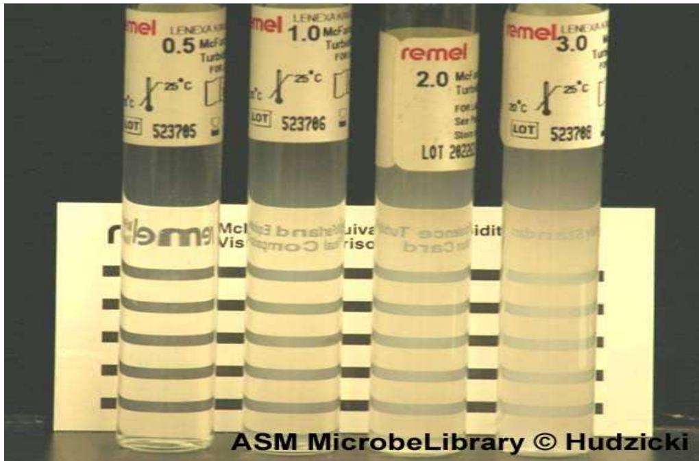
FIG.- 1.16. McFarland standards (left to right) 0.5, 1.0, 2.0, 3.0, positioned in front of a Wickerham card.
