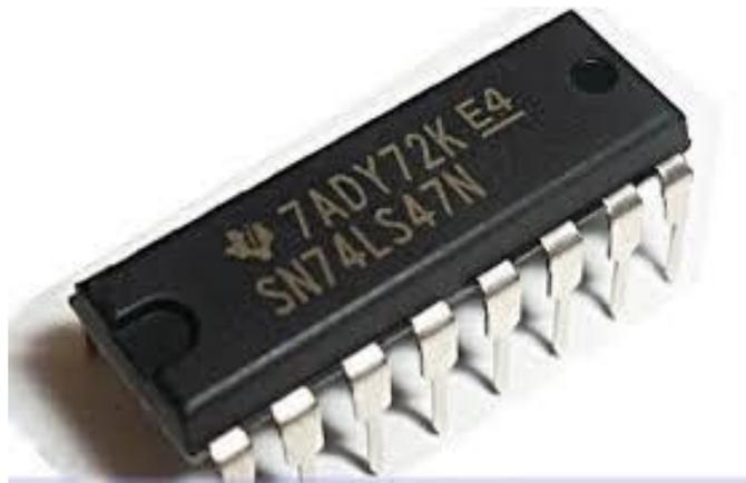
Fig 3.4.3: BCD to 7-segment display decoder driver
