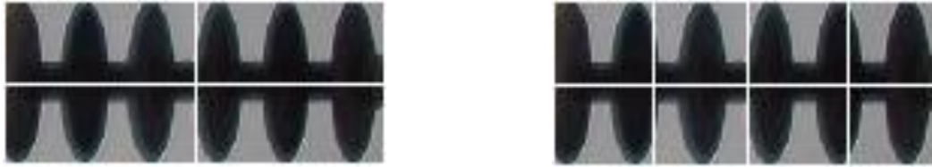
Figure 3.19: Left: An insulator image divided into 2 \times 2 sub-regions, Right: An insulator image divided into 2 \times 4 sub-regions
