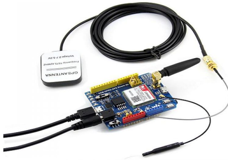
Figure 2.4: GSM/GPRS/GPS/Bluetooth SIM808 Shield (B) [7]
