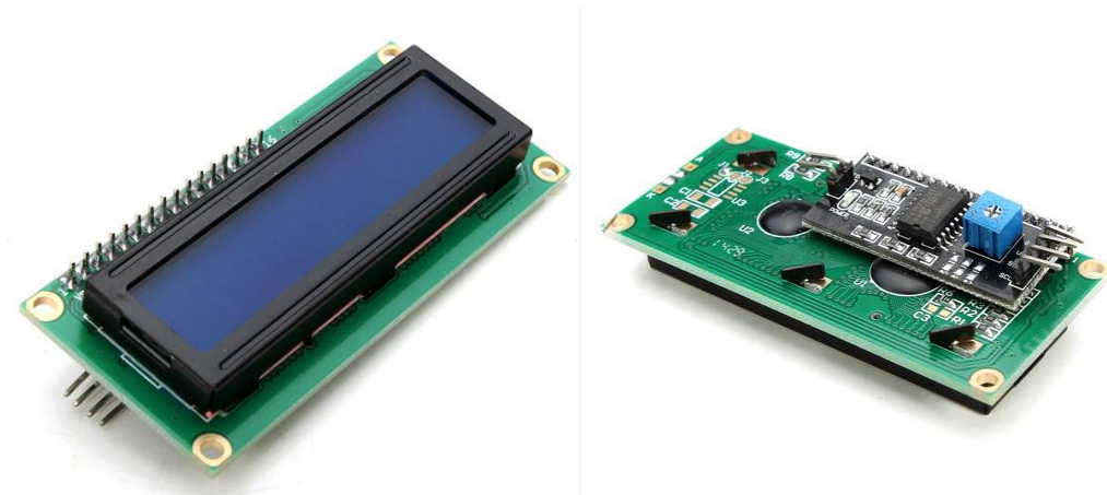
Figure 2.6: IIC / I2C 1602 Blue Backlight LCD Display Module[8]
