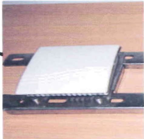
Figure 4.52: Temperature and Humidity sensor
