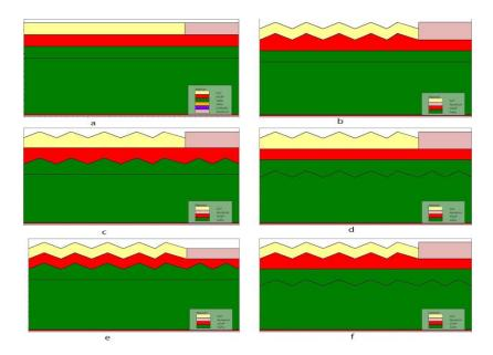
Figure-3.1: Structures of different solar cells having surface texturing on different regions.
