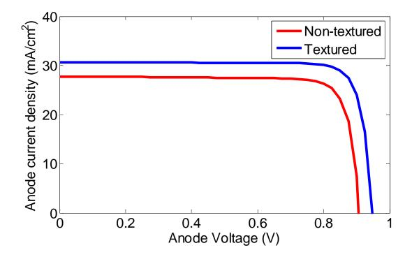
Figure-3.8: Anode current density versus anode voltage characteristics of non-textured solar cell and textured solar cell.
