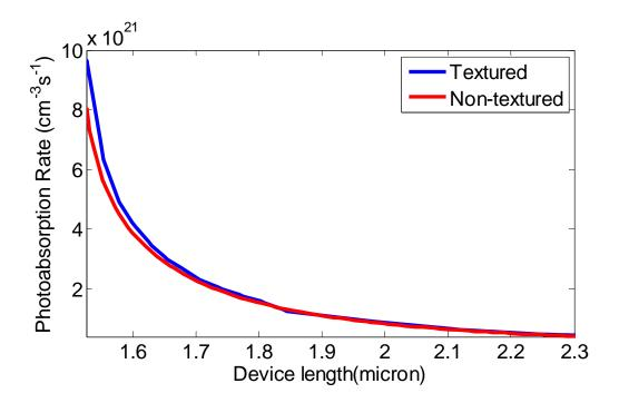
Figure-3.12: photon absorption rate versus device length (micron) of non-textured solar cell and textured solar cell.
