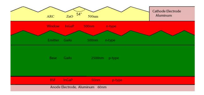
Figure 2.2: Textured single junction solar cell.
