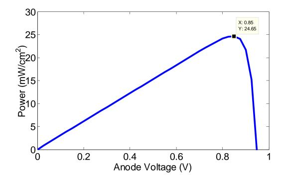
Figure-3.7: Power versus anode voltage of textured solar cell.
