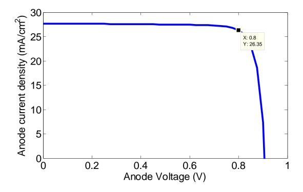
Figure-3.3: Anode current density versus anode voltage characteristics for non-textured solar cell.
