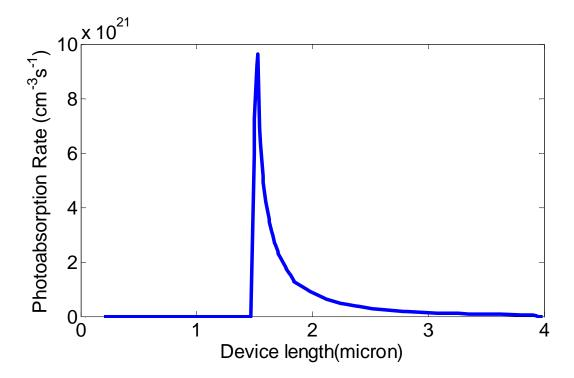
Figure-3.11: photon absorption rate versus device length (micron) of textured solar cell.
