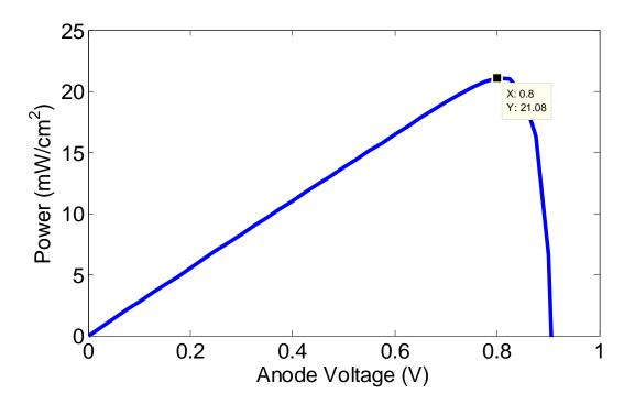
Figure-3.6: Power versus anode voltage of non-textured solar cell.
