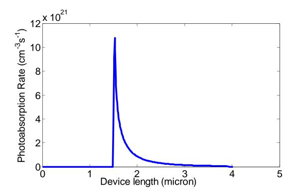
Figure-3.10: photon absorption rate versus device length (micron) of non-textured solar cell
