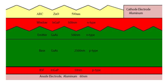
The structure of textured solar cell is given below in figure 3.4.
