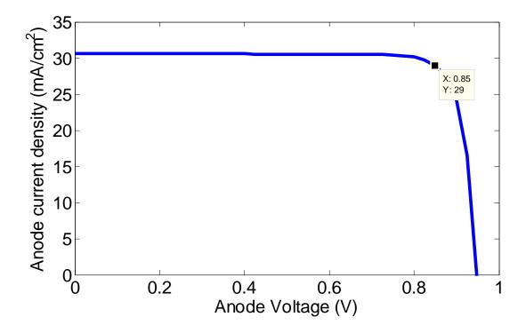
Figure-3.5: Anode current density versus anode voltage characteristics for textured solar cell.
