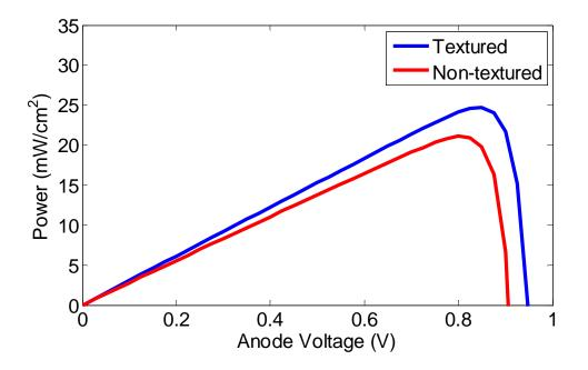
Figure-3.9: Power versus anode voltage of non-textured solar cell and textured solar cell.
