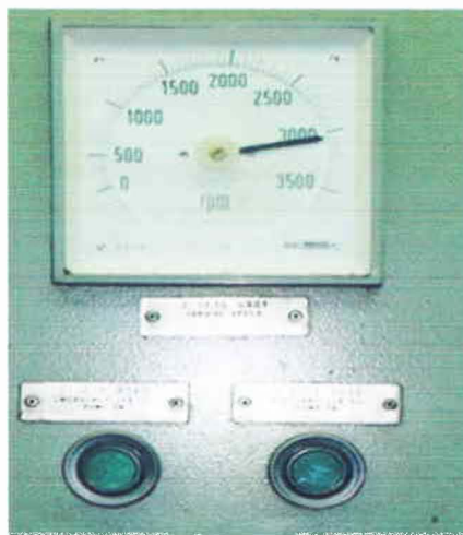
Figure 2.9: Speed of rotor checking (Tachometer)
