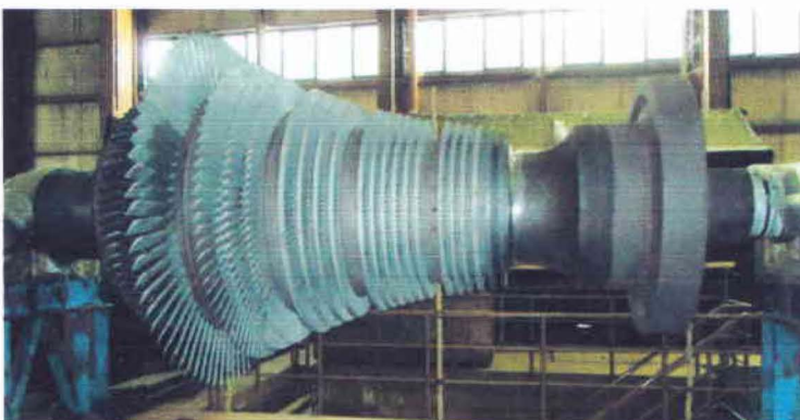
Figure 2.5: An Impulse turbine of unit 4 in APSCCL removed for overhauling
